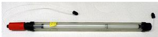
Figure 4.1 A size exclusion column
