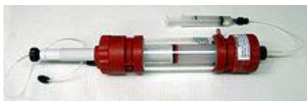
Figure 3.2 Preparative-scale ion exchange column used for protein purification
